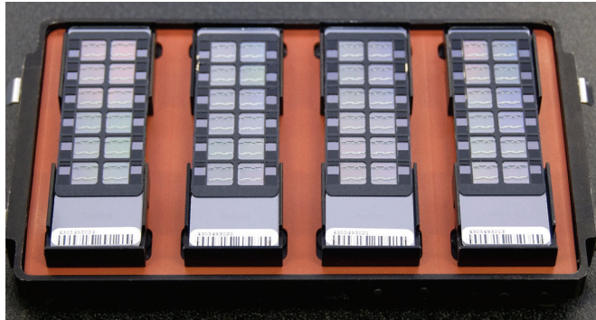
Figure 45 Placing Hyb Chamber Inserts into the Hyb Chamber
