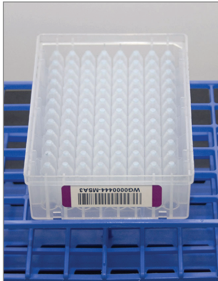
Figure 126 Uncovered MSA3 Plate Inverted for Air Drying
