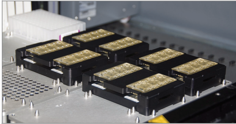
Figure 150 Full Set of Robot Tip Alignment Guides (Two Piece) on Robot Bed
