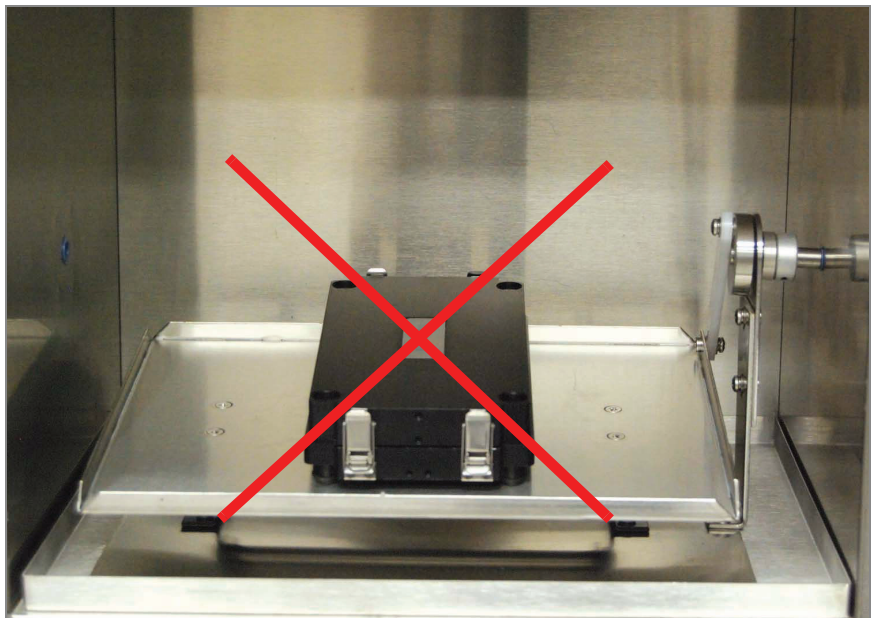
Figure 49 Incorrectly Placed Hyb Chamber
