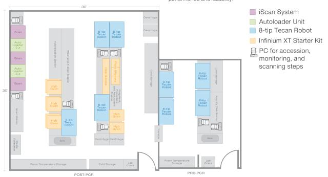
Figure 4: Example Lab Layout for Infinium XT Production-Scale Genotyping—An example lab layout is provided for processing 1,000,000+ samples per year and includes: three (8-tip) Tecan robots, three iScan Systems, two AutoLoader 2.x units, and ancillary lab equipment. This example layout requires approximately 1200 square feet. Layout is not to scale.
