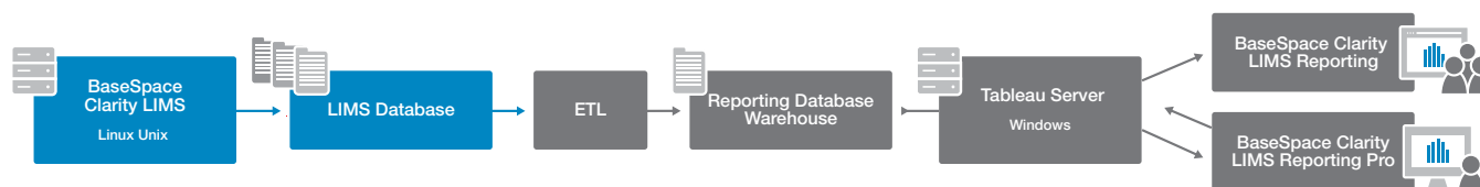
Figure 1: A High-Level View of the BaseSpace Clarity LIMS Reporting Architecture
