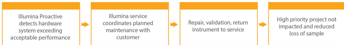
Figure 1: Example of how Illumina Proactive can benefit laboratories through detection of risk failure and facilitated troubleshooting —Routine monitoring of system performance data results in detection of failure risk for optical hardware, resulting in planned maintenance around a high priority project. A potentially expensive loss of time, effort, and sample is avoided.
