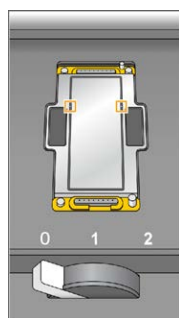
Figure 14 Inspect Vacuum Holes
