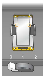
Figure 8 Inspect Vacuum Holes
