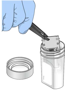
Figure 6 Remove Flow Cell
