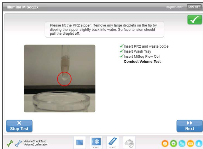
Figure 19 Remove Droplet from Sipper
